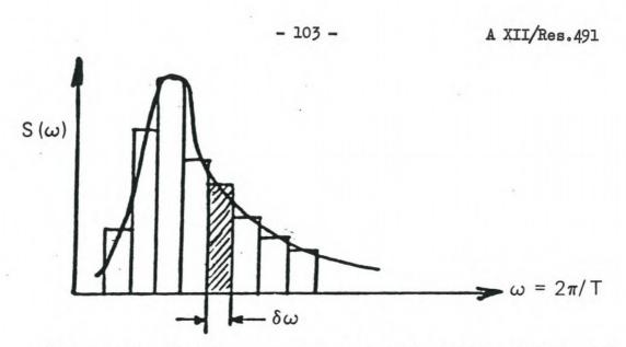
Each incremental area represents the wave energy in that incremental band of circular frequencies, i.e.  $dE = ggS(\omega_n) d\omega_n$ .
